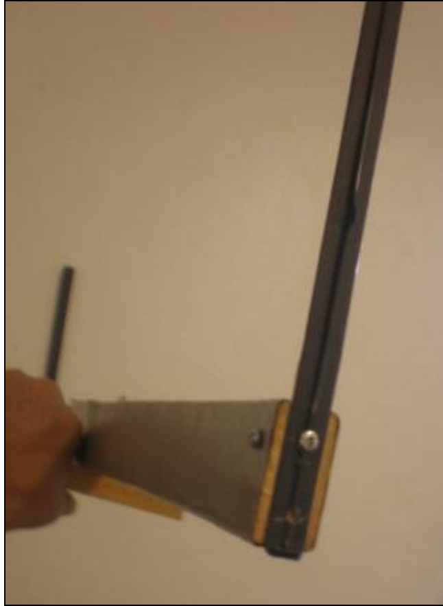
At Both Edges, Cross Section Distortion Prevented by a Piece of Wood Only Fastened at One Side with Centerline Guides for Measuring the Twist Angle
